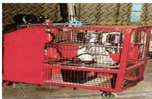
Figure 22. Hydrogen fuelled diesel Engine developed at IIT Delhi
